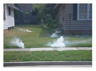
Smoke coming out of the ground may indicate a break or other defect in the sewer line which allows smoke to escape up through the ground.
